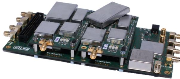
Figure 1.5: LDACS Receiver Hardware
