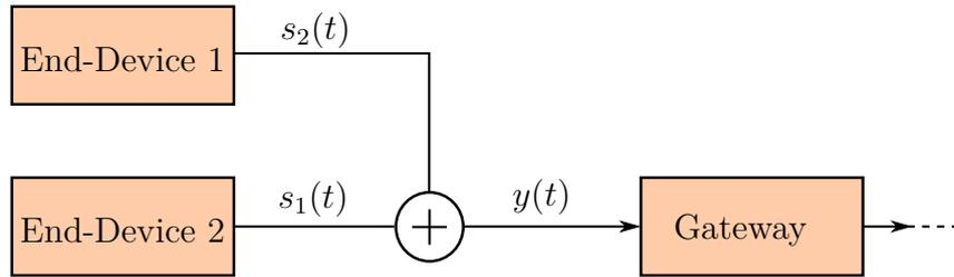
Figure 5.1: Scheme of the measurement setup with multiple LoRa signals
