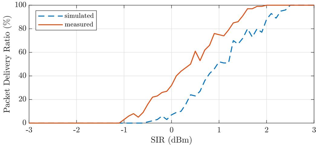
Figure 5.3: Packet delivery ratio over  $SIR$  of the first signal. Both LoRa signals with  $SF = 12$ ,  $BW = 125$  kHz, low data rate mode, payload length of 20 Bytes, and random delay uniformly distributed over signal length of the first signal.
