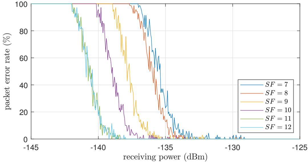
Figure 3.5: Sensitivity analysis; LoRa signal with bandwidth 125 kHz, code rate  $4/5$ , and different spreading factors; low data rate mode is enabled for signals with  $SF = 11$  and  $SF = 12$ .
