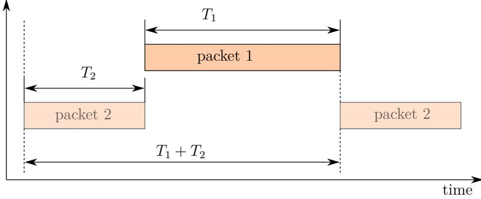
Figure 5.7: Collision of two LoRa packets at the receiver
