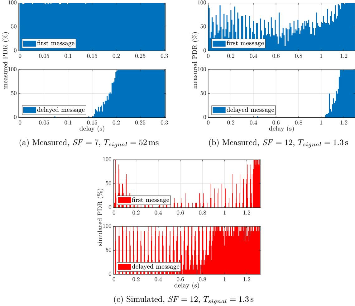
Figure 5.4: Packet delivery ratio of two delayed signals a) measured with both  $SF = 7$ , b) measured with both  $SF = 12$ , and c) simulated with both  $SF = 12$ ; Each signal with  $-100$  dBm receiving power,  $BW = 125$  kHz, and a payload length of 20 Bytes
