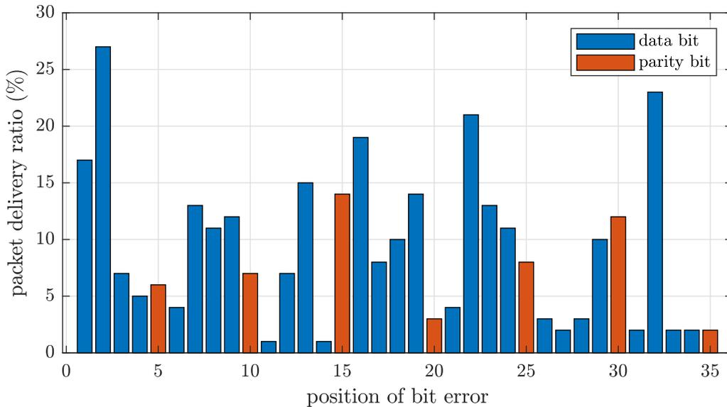
Figure 3.7: Reception of a erroneous signal with bit error at different positions after encoding step in section 2.1.4.1; signal with receiving power of  $-110\text{dBm}$ ,  $BW = 125\text{ kHz}$ ,  $SF = 7$ , payload length of 20 Byte, enabled CRC, and disabled low data rate mode.
