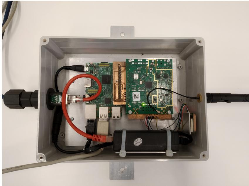
Figure 3.1: Gateway: Raspberry Pi 3 with IMST iC880A-SPI-LoRaWAN concentrator
