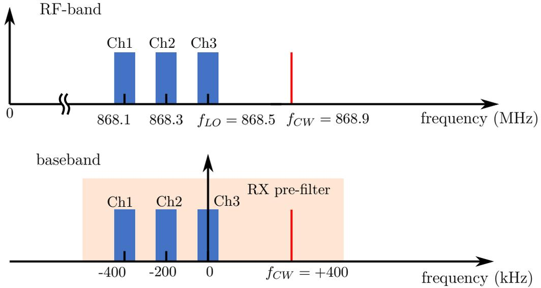
Figure 4.4: Spectrum in RF-band and baseband of the three mandatory channels with a CW interference
