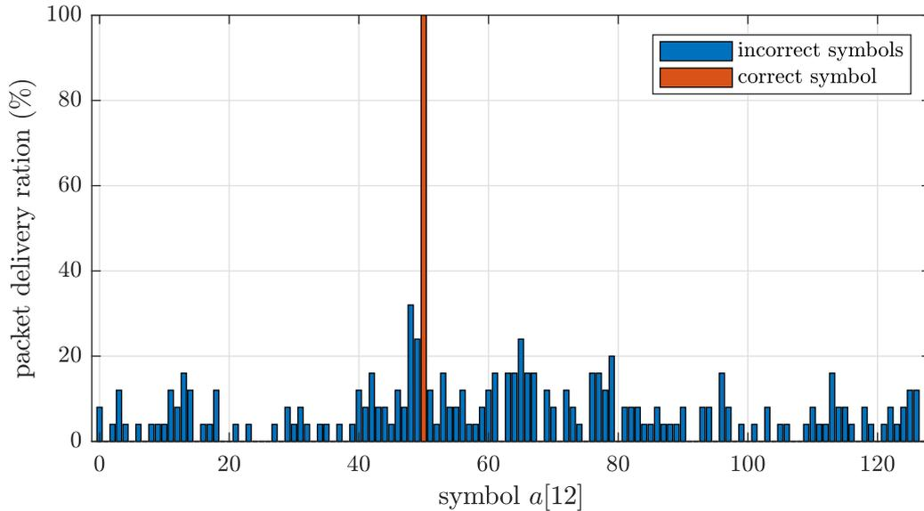
Figure 3.8: Packet Delivery Ratio over variation of symbol  $a[12]$ ; signal with receiving power of  $-110\text{dBm}$ ,  $BW = 125\text{ kHz}$ ,  $SF = 7$ , payload length of 20 Byte, enabled CRC, and disabled low data rate mode.
