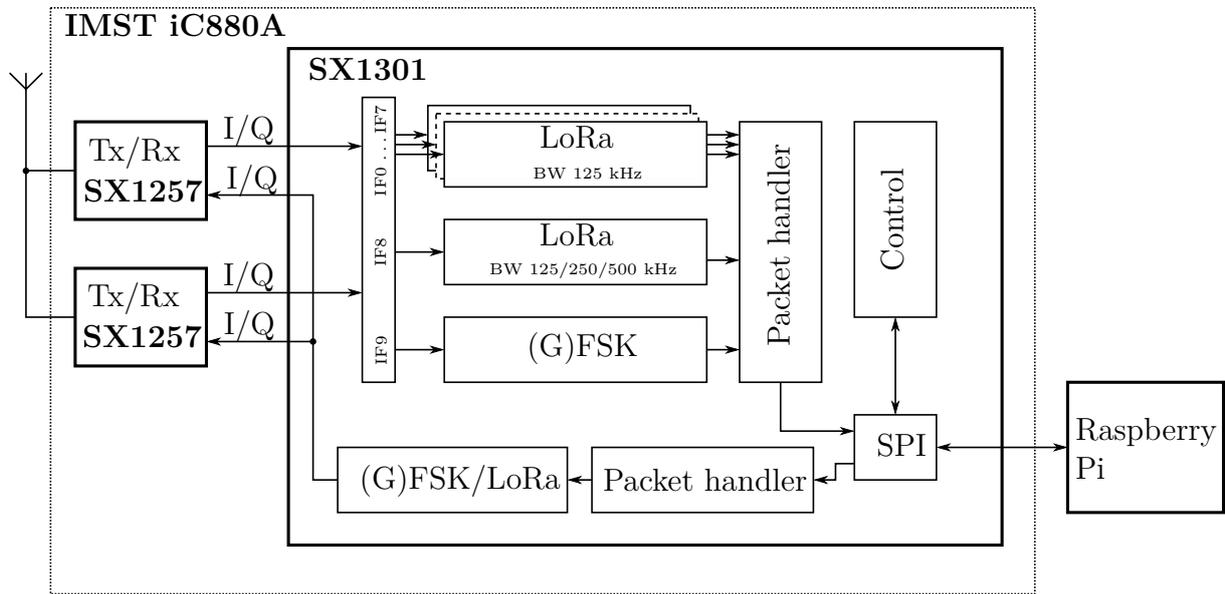
Figure 3.2: Block diagram of the IMST iC880A-SPI LoRaWAN concentrator [7]
