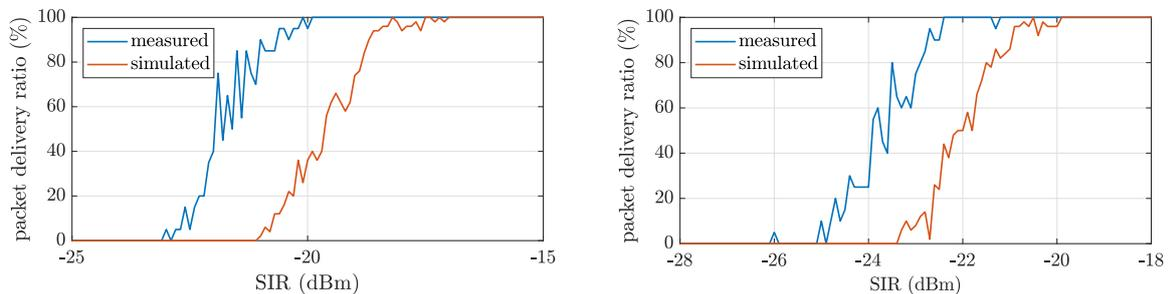
(a) Signal with  $SF = 11$ , interfering signal with  $SF_{int} = 12$
